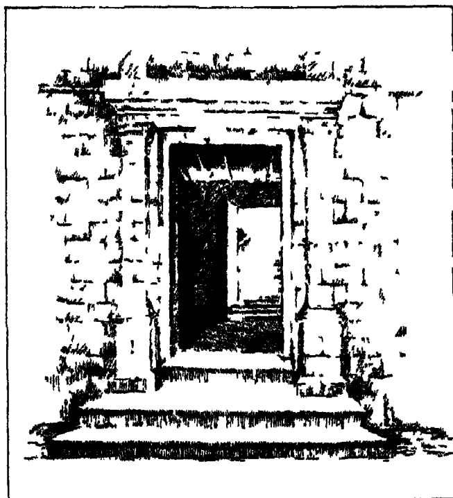
STEEL DOORWAY IN WHITE PORTLAND CEMENT
