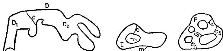
FIG. 12.— D is a simply connected region. E is twofold connected. F is fivefold connected.
